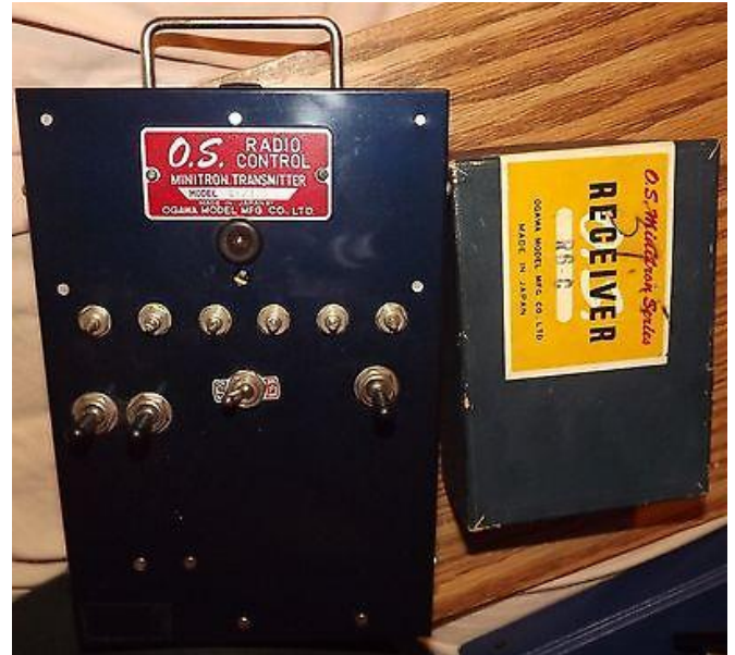
Typical 6-channel reed type transmitter and receiver. This would be equivalent to a 3-channel modern radio. You needed two channels for every control surface, one to move the servo left, and one to move to the right.
